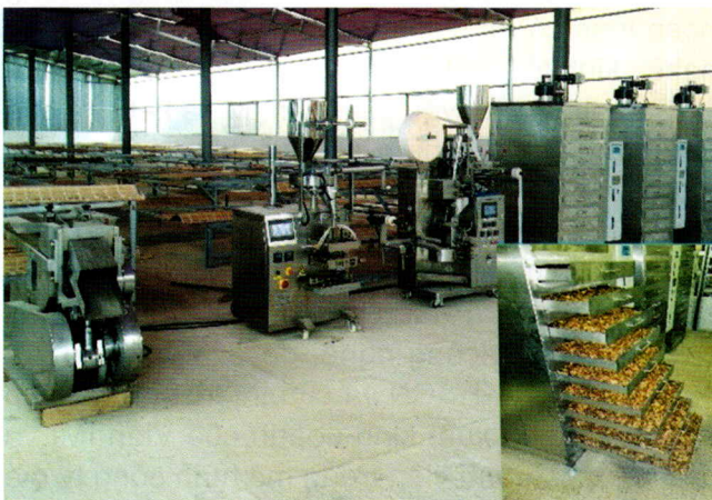
System of equipment for preliminary processing of raw materials, packaging machines and automatic infrared drying oven for medicinal herbs manufactured by IMI Institute.
